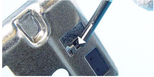
28.) Release the snap of Earpiece Connector by using the slotted screwdriver.
