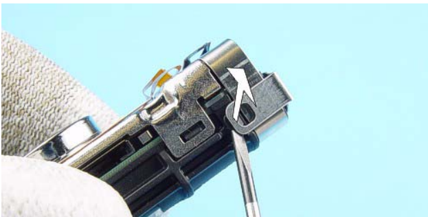
11.) Use a slotted screwdriver to lift the Battery Lock .
