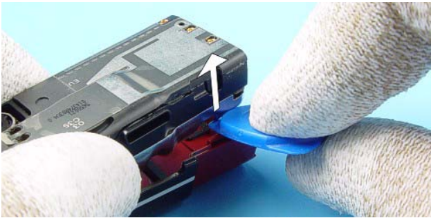
9.) Lift the modules from the B-Cover by using SRT-6.
