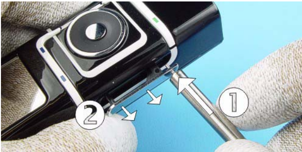
1.) Use the SIM tray release tool to open the SIM Holder .
